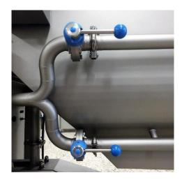
All piping parts can be dismantled very quickly - and without tools - by means of triclamps. They have no screw thread on the pipe-ends, and because of that they are much more hygienic than the common used dairy fittings (nut/coupling nut).
