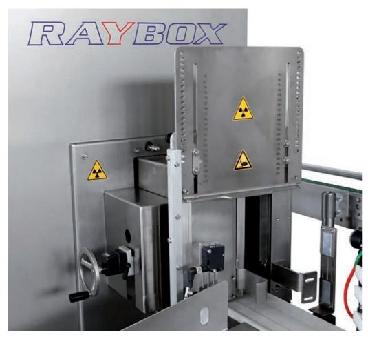
Automatic check of the protective screens and beam-traps position. If those devices are in the wrong position the machine does not run.
