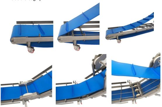
The upper belt can be pushed out of the front workstation after the power plug has been removed from the socket. The turning roll can be released by pressing only one button. The belt can then be removed from the frame so that the belt frame can be cleaned.
