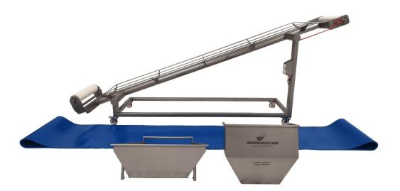
• The belt can be cleaned thoroughly and easily. The input and output funnel can be detached very easily. By means of a unbolt button, the turning roll can be turned over to release the belt. Because the frame only has legs on one side, the belt can be removed from the belt frame on the other side very easily. Another advantage is that the belt frame can be cleaned perfectly on the inside as well.
