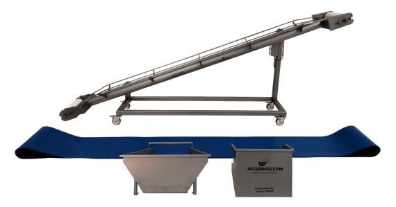
• The belt can be cleaned thoroughly and easily. The input and output funnel can be detached very easily. By means of a unbolt button, the turning roll can be turned over to release the belt. Because the frame only has legs on one side, the belt can be removed from the belt frame on the other side very easily. Another advantage is that the belt frame can be cleaned perfectly on the inside as well.
